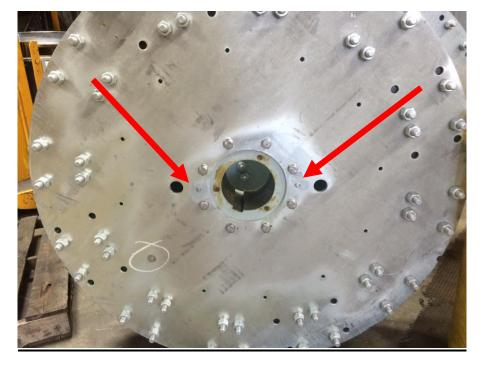
Install 2 pins on top and 2 pins on bottom of hub as shown in above example
